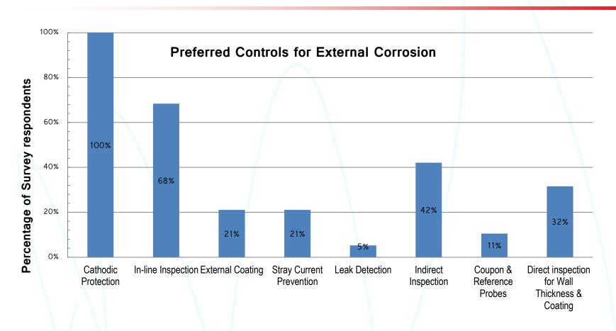
**Control Mechanisms for External Corrosion**
